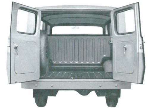
Two full swing-out doors which close at the center facilitates access of personnel and make loading easier.
