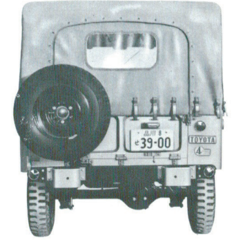
Roll-up type rear curtain together with a drop-gate
