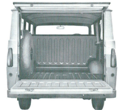
With the lift gate up and tail gate dropped level with the floor, additional cargo area is provided.
