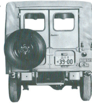
Canvas and steel gates swinging out at the center
