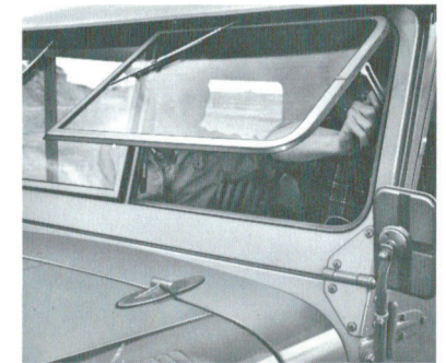
PUSH-AND-OPEN TYPE WINDSHIELD A top-hinged windshield that may be opened from the bottom is available as an optional item. (optional extra)
