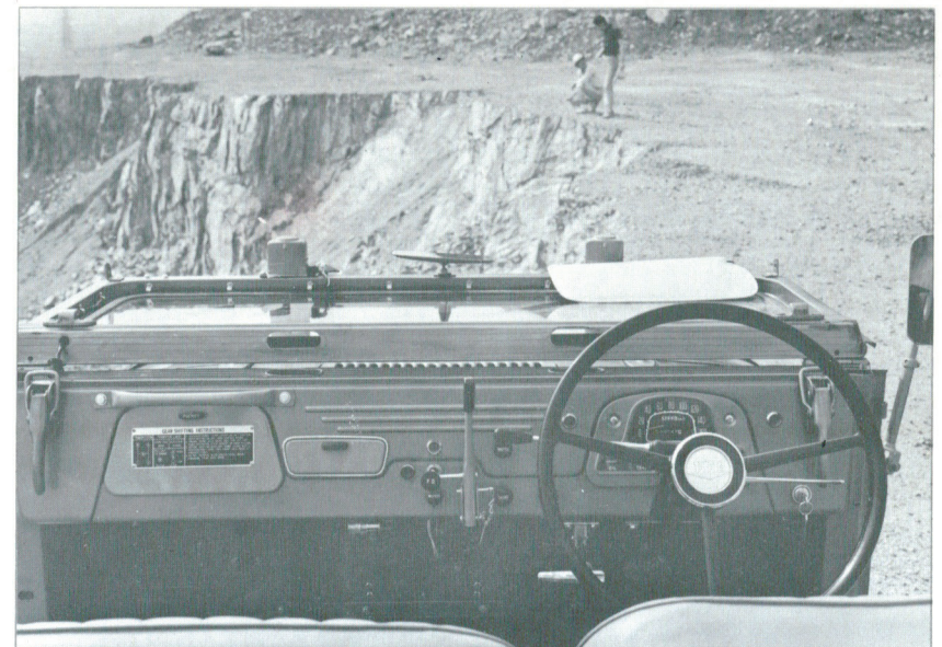
PUSH-AND-OPEN TYPE WINDSHIELD A top-hinged windshield that may be opened from the bottom is available as an optional item. (optional extra)
